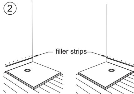
2 Secure the filler strip to fill the redundant rebate.
