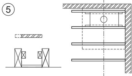
5 Place the supplied plywood waste support over the position of the waste outlet. Cut to fit between the joists. Support on 2 number 50mm x 25mm battens screwed to the sides of the joists. Ensure the waste support is level with the top of the joists.
