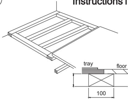
Follow previous instructions 1-4. Secure battens to the subfloor @ 400mm centres and around the perimeter of the tray.
