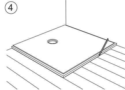
4 With the tray on the floor mark its position with a pencil. Move the tray aside and then remove the floorboards.
