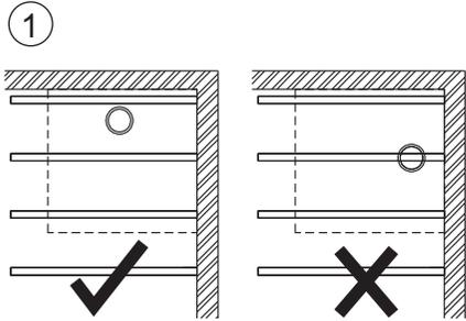
1 Locate the position of the shower area. Place the tray on the floor. Position the waste outlet hole so that it is not obstructed by any of the joists.
