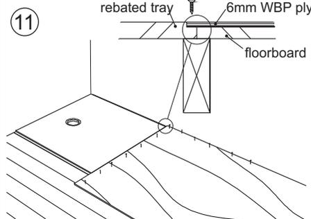
11 With the tray and all the flooring secured, line the rest of the floor with 6mm WBP ply. Pin and glue or screw plywood into the rebates. Sand level.
