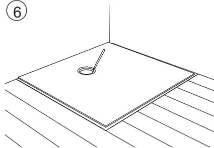
6 Place the tray in position and mark out the hole for the waste on the waste support plywood. Remove the tray and cut out the hole.
