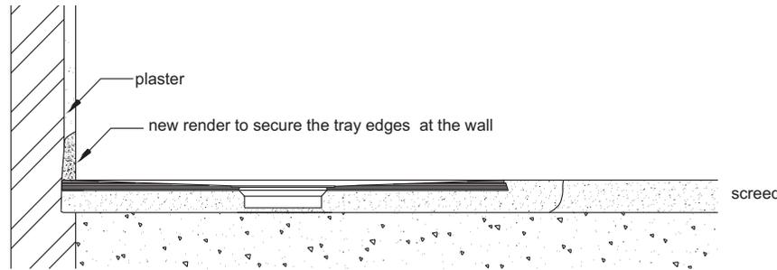
The tray assembly can then be bedded down on a mortar bed, ensuring the waste is fully supported. Screed up to the external edges, where the tray is against the wall, make good the wall and plaster down onto the tray.
