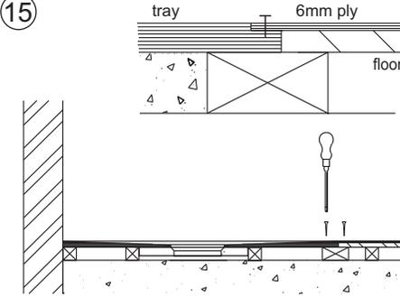
Secure the tray to the battens using 50mm No 8 countersunk wood screws @ 225mm centres.
