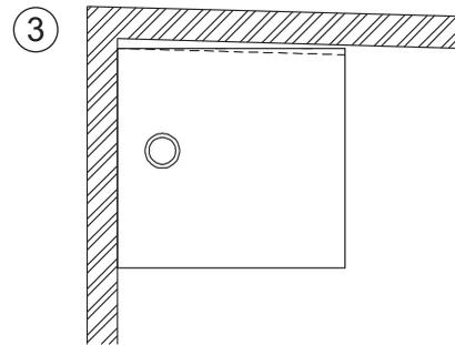
3 Place the tray into the corner. Scribe and cut to shape if necessary.
