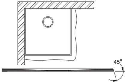
Hack up the floor screed to suit the tray size. Cut off the exposed rebated edges on the tray at 45°
