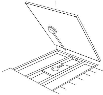
With the shallow waste installed into the tray and the waste support secured to the battens, place the tray into position.
