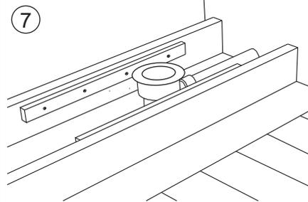
7 Position the waste pipe to a suitable drain, including where necessary forming a hole in the wall. Remove the trap. If using a TS52-116 once in position, connect the lower section of the trap to the waste pipe
