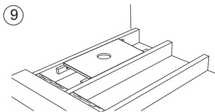
9 Place tray in position. BEFORE FIXING THE TRAY MAKE SURE IT IS LEVEL ON ALL SIDES. Install the trap as per manufacturers instructions.
