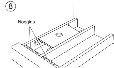
8 Secure the waste support to the battens. Install noggins between joists to support the tray where necessary.
