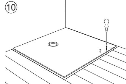
10 Secure the tray to the joists using 50mm x No 8 countersunk screws @ 225mm centres.
