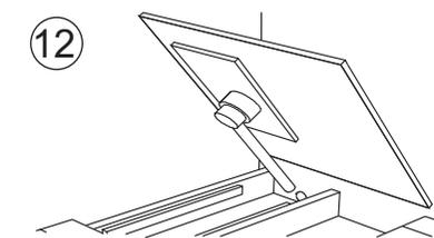
12 Where it is difficult connecting the waste pipe, unscrew the tray and waste supports, replace both sections, screw the tray to the waste support, lift out, make up waste pipe and trap. Line up waste pipe and slide into position. Secure as before.
