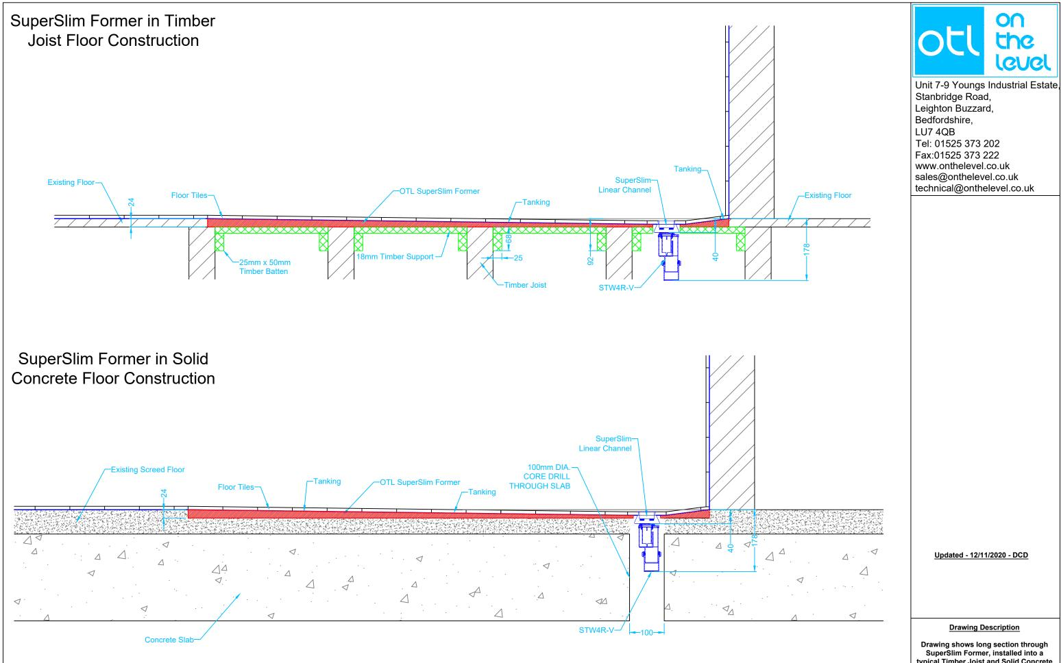
typical Timber Joist and Solid Concrete floor construction.
