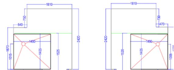
On The Level manufactured the whole bathroom floor with falls incorporated in the shower areas. All complete wet room floors were provided to RGB Group in two sections for ease of installation.
