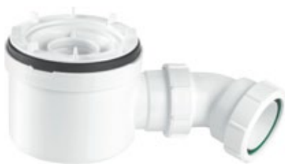
OTL REF: OTL ST90-HPB 50mm Water Seal Trap Body with 2" Multifit Outlet. Overall height with Tile 120mm. Flow rate 50 l/min. (Flow rate calculated under a constant 15mm head of water)
