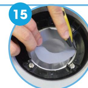
With a knife cut away the excess matting inside the clamping ring
